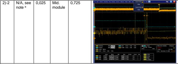
Note: the voltage across the arc is too low, the disconnection should be caused by loss of PV supply due to DC converter disconnected.
