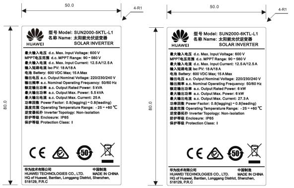
Note: inverter marking only, a seperated marking regarding to arcing characteristic should be provided on inverter as well according to draft standard IEC 63027 ED1, 82/1636/CDV
