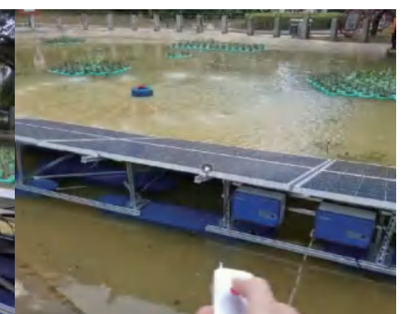
System: 2 sets 750W solar aeration system Location: Shenzhen
