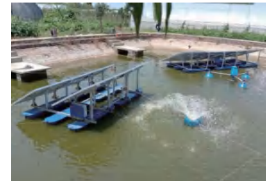
System: 1.1kW & solar aeration system Location: Hefei
